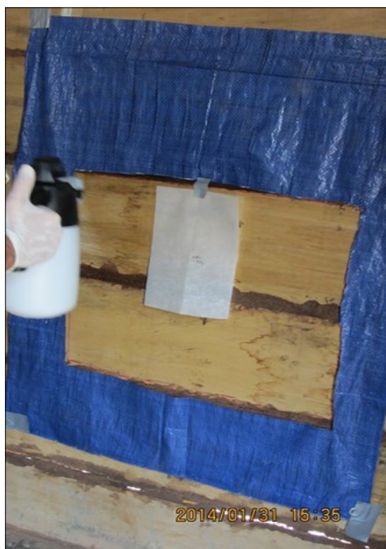
Fig 2. Applying insecticide with a flat fan, small volume sprayer on the wall field limited by a hollid tarpaulin frame and with a Whatman paper attached at the middle of the spray field for collecting spray data.
